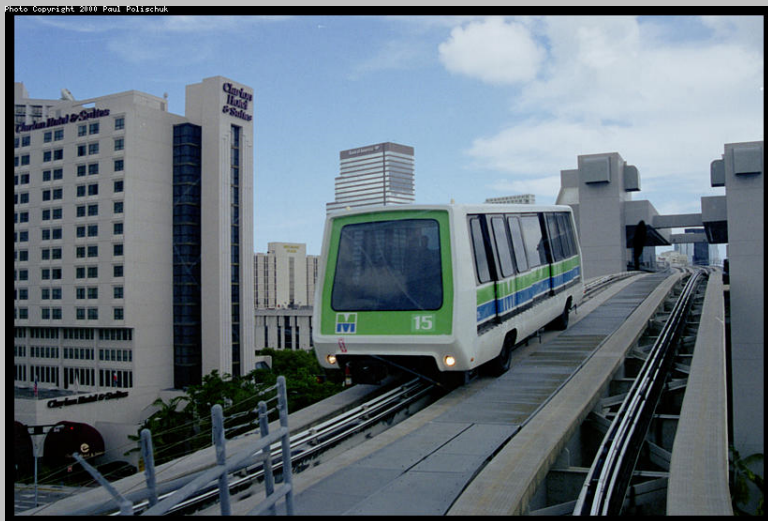
Metromover is a free automated people-mover system that serves downtown Miami. Photo: Paul Polischuk
